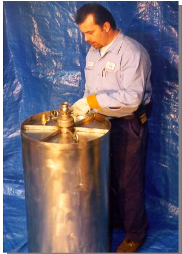
SCF-7 Canister Holds 7 Filter Elements
