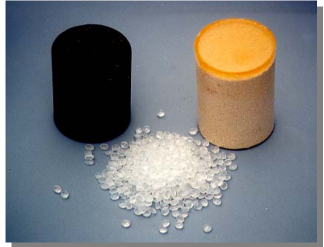
Polymer-solidified Waste Samples
